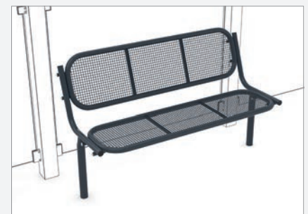
Bench U-2010 Bench with continuous seat surface and backrest made of wire mesh. The bench is prepared for free-standing installation, alternatively with leg extension for paving over. The design is hot-dip galvanised and powder-coated according to RAL. Grid dimension 1500 mm.
